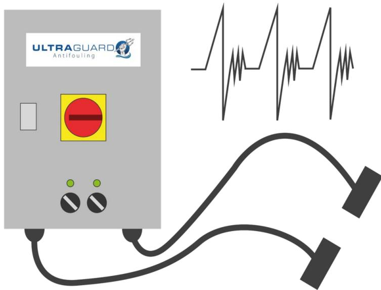
By causing each transducer to resonate at the correct frequency we induce the required vibrations which prevent the larvae from attaching themselves to the surface being protected.
